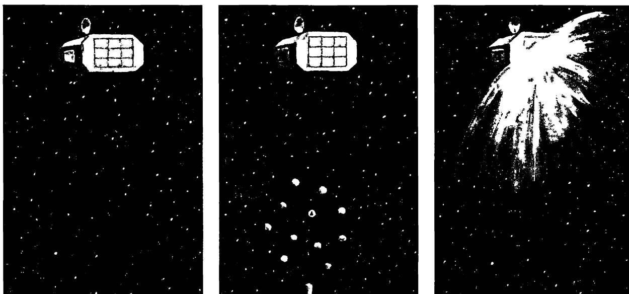
Rocket Attack: Ground-based rockets could attack defense satellites, releasing a homing warhead and a cloud of decoys to make the antisatellite (ASAT) weapon difficult to intercept. Future ASATs may also be fast-burning and maneuverable, yet are likely to be substantially cheaper than defense satellites.
